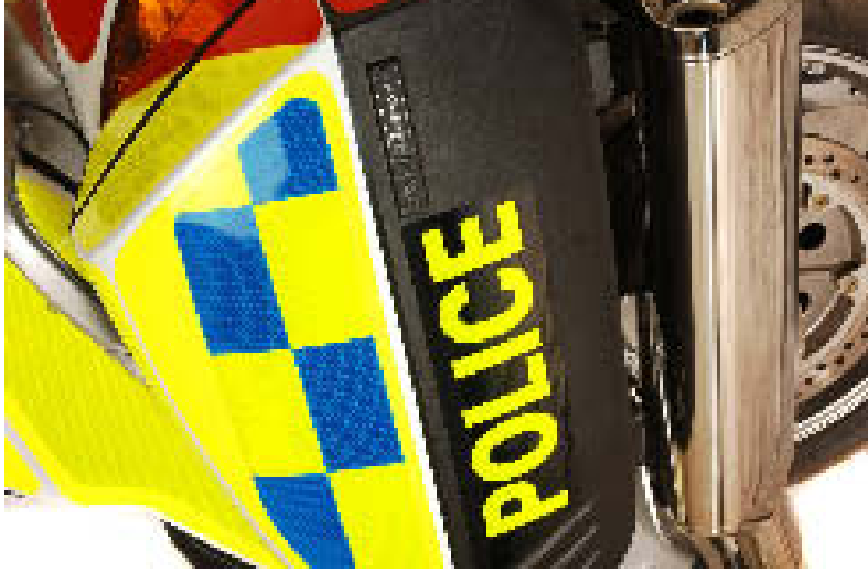
Photograph 11. Detail of pannier area, showing recommended arrangement of POLICE legend
