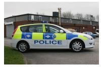
Nikkalite® Flexible Crystal Grade retroreflective and fluorescent retroreflective liveries are very conspicuous providing early recognition of the vehicles position to other road users due to;
