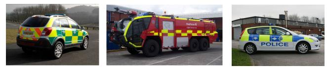
Nikkalite® Flexible Crystal Grade retroreflective and fluorescent retroreflective liveries are very conspicuous providing early recognition of the vehicles position to other road users due to;
